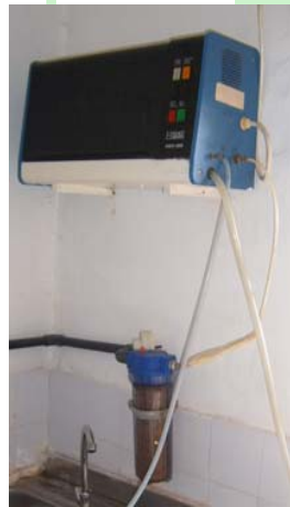
Water distillation system
